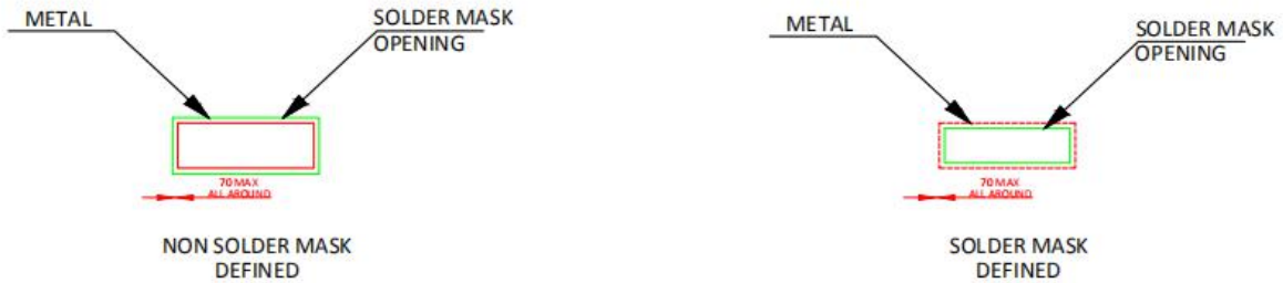
Figure 9.2 SOW8 Package Board Layout Example
